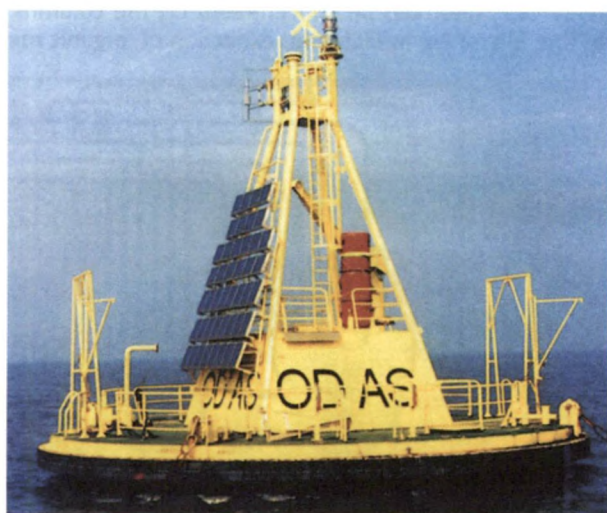
Figure 5.1b Discoid buoy 'META-1' The buoy has a diameter of 12m and a draught of 1.6m. It is fitted with solar panels and a diesel generator. The sensors are installed in a sensor frame underneath the bottom of the buoy in a depth of about 2m. Access to the sensors is via a moon-pool of about 70cm diameter. On the mast navigational lights, antennae and meteorological sensors are installed. The buoy is located in the salinity gradient of the Elbe in front of the Kiel canal near Brunsbüttel.
