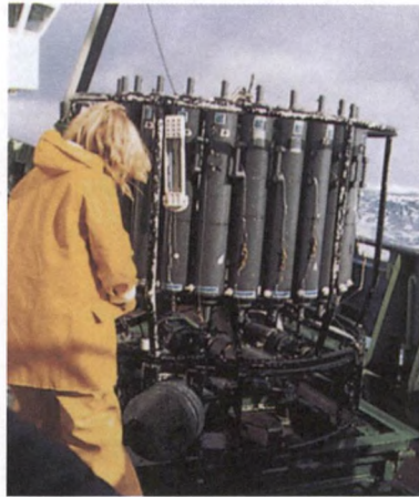
Figure 4.3 Deployment of a conductivity, temperature and depth (CTD) sensor rosette array at sea Source: SOC
