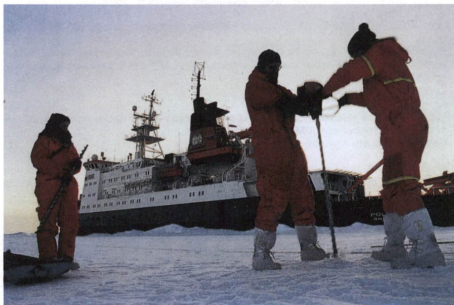
Figure 6.2 Drilling to measure the thickness of the marine ice and to recover samples, North Polar Sea Source: H Grobe, Alfred Wegener Institute for Polar and Marine Research, Bremerhaven
