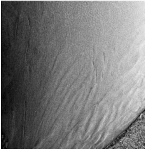
Figure 8: A typical SAR scene illustrating the surface expression of bathymetric features (supplied by ARGOSS)
