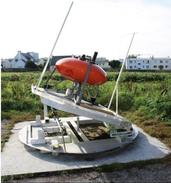
Fig. 1. Picture of the calibration platform for compass and tilt sensors. Current-meters and current profilers can be calibrated with their instrumented mooring cages to take into account the instrumental error.
