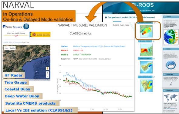
Fig. 2. Snapshot of the Multi-parametric Ocean Model Skill Assessment tool, implemented by PdE to validate operationally SAMOA downscaled local solutions and to compare them with the “parent” regional solution in which are nested (the CEMES IBI MFC forecast product).
