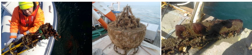
Fig. 2. Bio-fouling of in situ sensors after three months.
