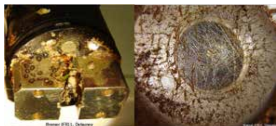
Figure 3 Biofouling effect on optical sensors.
