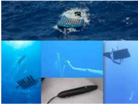
Figure 2 Detail of the Wave Glider with a towed array of hydrophones (towfish), attached to the submerged module.
