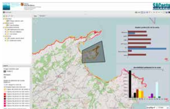
Figure 3 SACosta tool applied to the northeastern coast of Mallorca: an automatic report of the coastline sensitivity and its degree of protection is generated for the shaded polygon drawn by the user.
