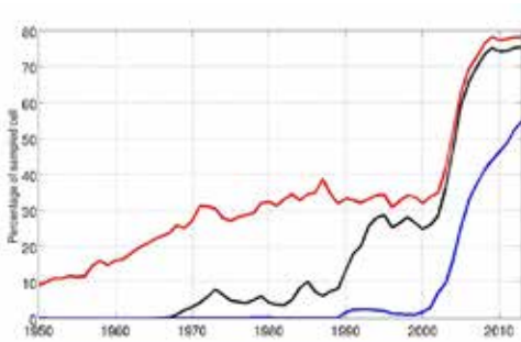
Figure 5 Percentage of 4 degree squares ocean cell sampled by at least one temperature sample between 0 and 50m depth (red), between 500m and 550m depth (black) and between 1500m and 1550m depth (blue).
