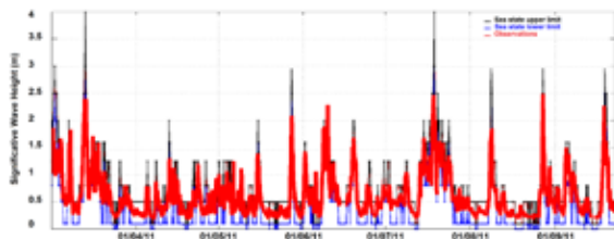
Figure 1. Time-series of in situ sea wave observations (red line) compared with the upper (black line) and lower (blu line) limit of the corresponding Wave Watch III model forecasts.
