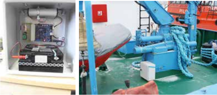
Figure 1 Instrumentation for ship hull vibration measurements as installed aboard EVA 316 (the instrumentation box before installation (upper panel) and after installation (lower panel)).
