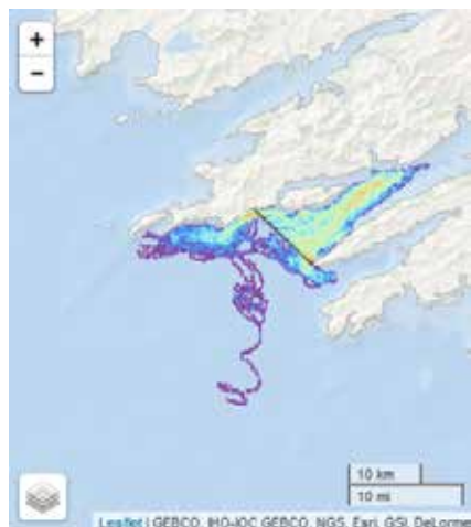
Figure 5 The particle-hours map from the 3-day forecast starting on 14 May 2014. Particles were released at the bottom layer along the transect shown. Colour scheme: purple – low values, orange – high values.
