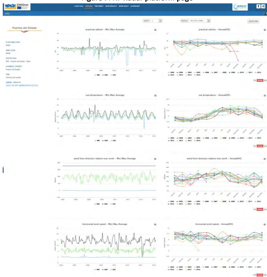
Figure 8. Example of the monthly synthetic data from the EMODnet Physics (platform 62084) - http://www.emodnet-physics.eu/map/platinfo/pimeanmaxmin.aspx?platformid=7340 . Once the monthly file is available, the system also supplies synthetic data (i.e. average, maximum and minimum) for the available parameters.
