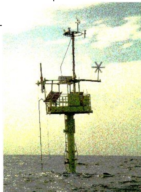
Figure 15. Institute of Baltic Sea Research, Warnemünde operates fixed monitoring stations in the Baltic Sea. These stations will extend the German Fixed Monitoring Network with on-line satellite data transmission to the central data base on shore. These stations are important to the permanent observation of the water exchange between the Baltic Sea and the North Sea, as well as the exchange between different shallow basins and the central Baltic
