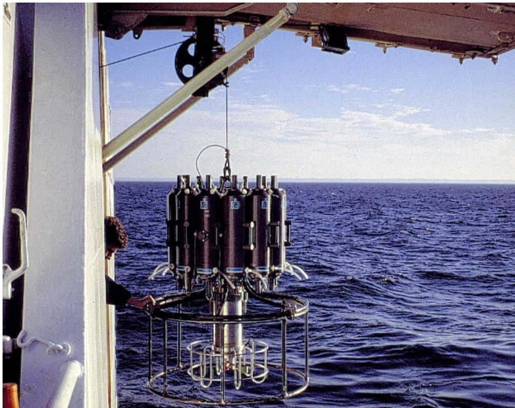
Figure 7. Environmental monitoring off Poland, showing use of CTD and rosette of water sample bottles
