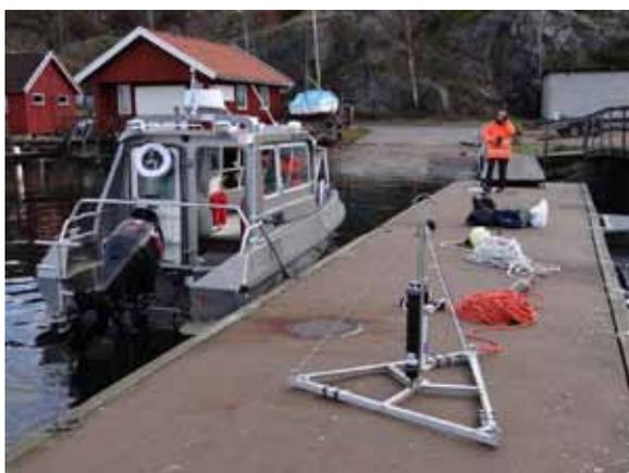
Figure 1. A seafloor system including the complete "U system" for anchoring, designed for a depth of 40 metres and ready for deployment. SMHI's "Sensorita" is shown to the left. Photo: Henrik Lindh
