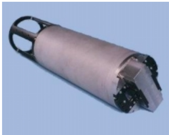
Figure 4. Fast Tracka. Fast repetition rate fluorimeter. Chelsea Instruments.
