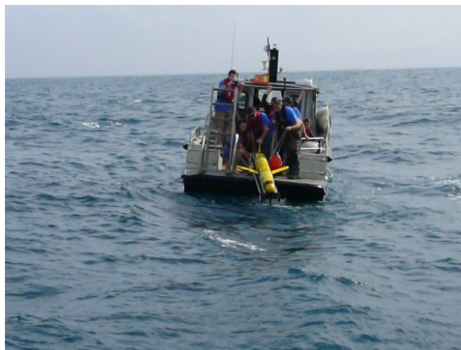
Figure 2. Deploying a Slocum glider in the field experiment of the PLOCAN glider school in 23. October 2015.
