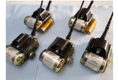
Animal Borne Ocean Sensors - oxygen sensor (CNRS)
