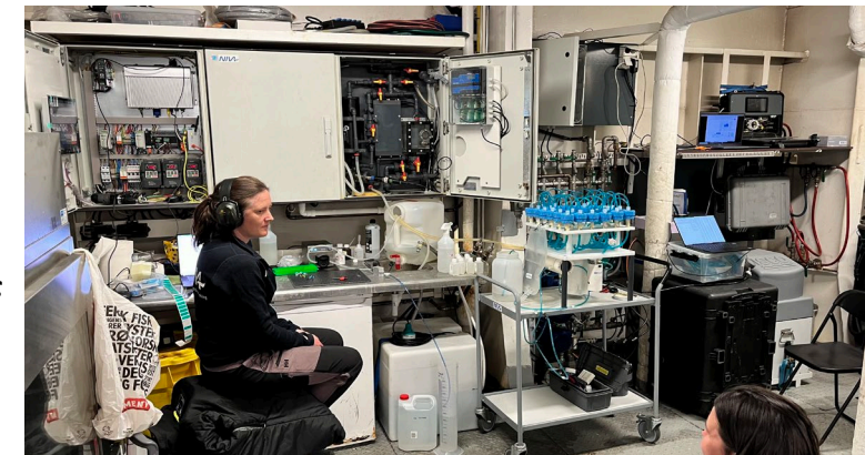
Particulate matter/eDNA sampler on M/S Trollfjord. Source: A. King, NIVA
