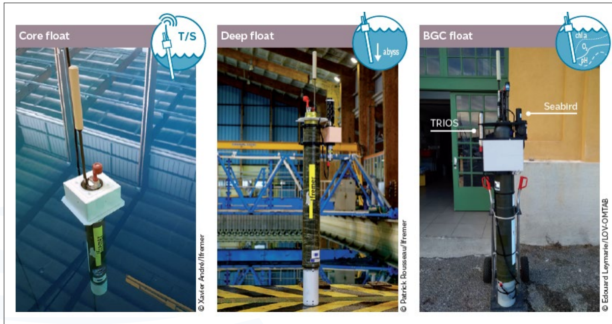
Figure 1. From left to right: Test of the RBR CTD on the Arvor float for the core mission, the two-head prototype to compare the SBE61 and RBR concerto new sensor for the deep mission, and the double irradiance sensor prototype to test TriOS vs Seabird for the BGC mission.
