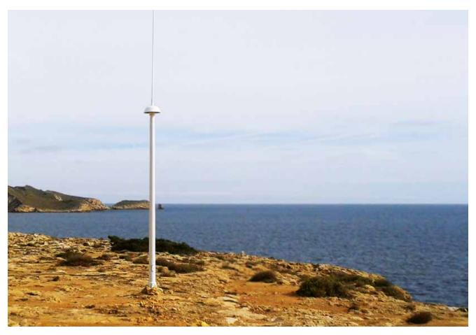
High Frequency radars collect real-time data on surface currents and waves © ICTS SOCIB
