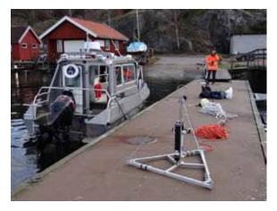
Figure 1. A seafloor system including the complete "U system" for anchoring, designed for a depth of 40 metres and ready for deployment. SMHI's "Sensorita" is shown to the left. Photo: Henrik Lindh
