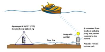
Figure 5. Anchoring on a muddy or uneven sea floor.
