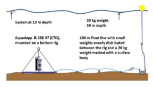
Figure 2. Anchoring with a surface buoy
