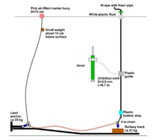
Figure 3. Anchoring system for the profiling float during tests in December 2014 in the Stockholm archipelago (depth 46 m).
