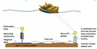
Figure 4. Anchoring with an Acoustic Release instead of a surface marker
